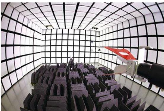
Figure 2-3. EMC Testing Chamber
