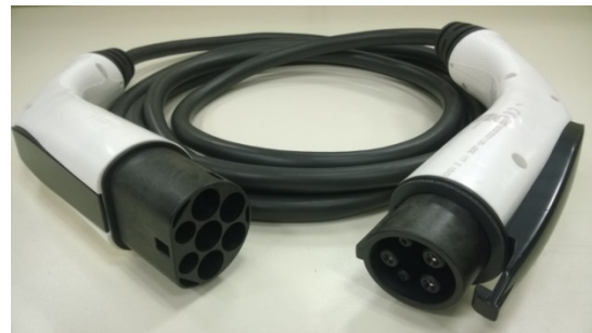
Figure 4-7 Conversion cable assembly type 1 (EV) – type 2 (EVSE)
