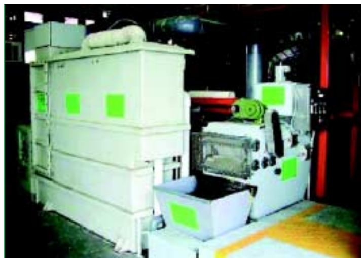
生產力局開發的「易浮」(E-FLOT)，是一套以電絮凝法為基礎的污水處理系統，可幫助除去食肆污水中的乳化油。 The E-FLOT developed by HKPC is an electro-flocculation system that can help remove emulsified oil in restaurant wastewater.
