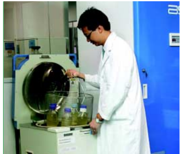
生產力局用高溫消毒爐協助客戶在進行微生物測試時，消毒盛載水質樣本之器具。 The Autoclave is used by HKPC to help clients disinfect glassware that holds water samples for microbiological tests.
